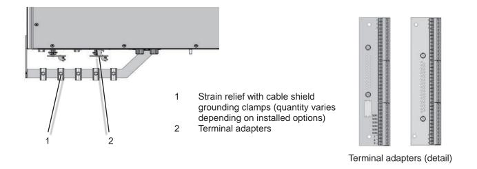
Fig. 2-7: X-STREAM X2GP - Signal Connections With Screw-Type Terminal Adapters (top View)
